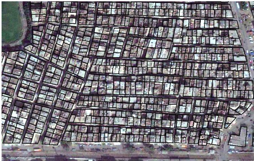
Figure (4.25): On Screen Digitizing for GEO EYE Satellite Image Extracted from Google Earth Program for Buildings.
